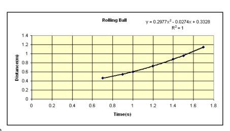
Notice that the relationship is indeed quadratic, with an excellent coefficient of determination. The usual methods of analysis yield an average accleration of  $0.60 \text{ m/s}^2$  for the rolling ball. A little trigonometry lets us calculate the value of  $g = 6.5 \text{ m/s}^2$ , certainly less than the accepted value.
